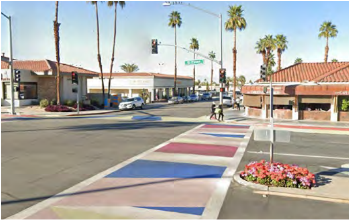
Highly-visible crosswalk art cues drivers to slow down, and indicates that the area is pedestrian-oriented.
