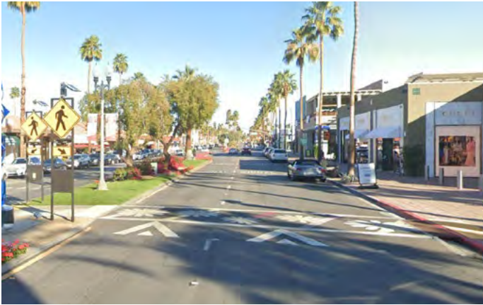
A painted, raised crosswalk is highly-visible, provides safer and accessible crossing conditions for pedestrians.
